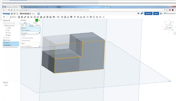
Use the Extrude tool again. This time, click on “Remove” in the Extrude options panel, and change it from “Blind” to “Through all”.
