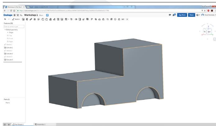
Use the Extrude tool again to cut both of these circles out to a depth of 5mm.
