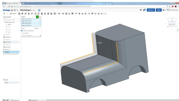
Click the “Fillet” tool on the Main Tool Bar. It’s a cube with a rounded edge.
