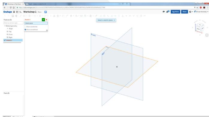
The functionality of CAD programs relies on creating “Sketches” and using various tools to either add or remove a solid object in reference to them.
