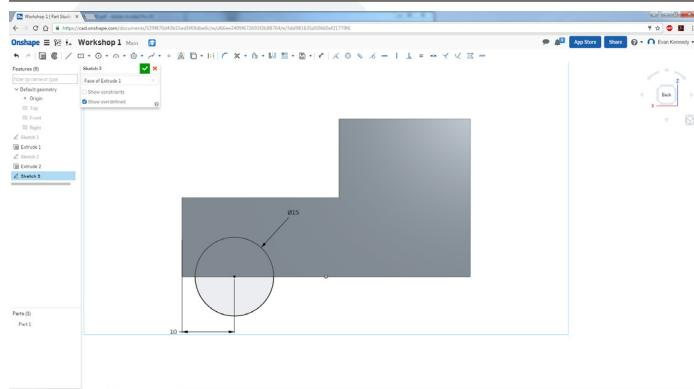
Make a new sketch on the same side. Draw a circle using the “Centre point circle” tool, that attaches to the bottom edge of your shape. Use the dimension tool to set the distance between the circles center point, and the left hand edge of your shape to 10mm (make sure you select the circle’s center point, not the circle itself).
