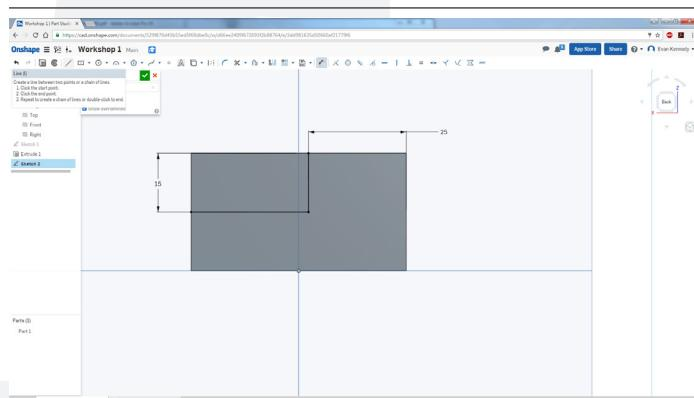
Create a new sketch on one of the large side faces of your box, and use the line tool to draw a shape like the one pictured here.
