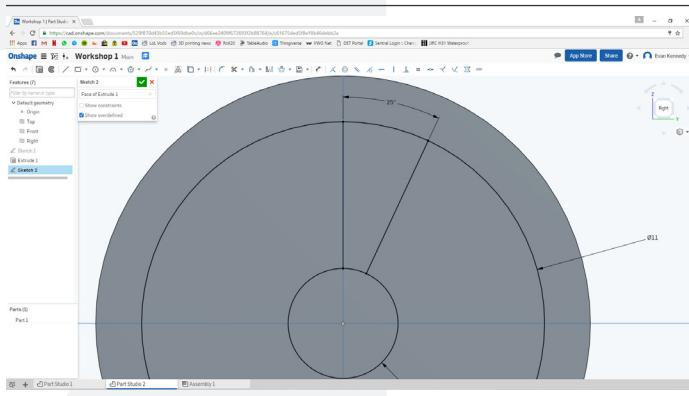
Draw a line from the top/center of the smaller circle, to the top/center of the larger one.
