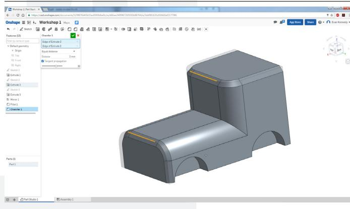
Similar to above, let’s use the Chamfer tool (next to the Fillet tool) to angle some edges.
