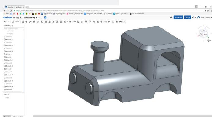
I've added headlights. 6mm diameter. 1mm depth. They share the centre point with the curved corners of the front of the train.
