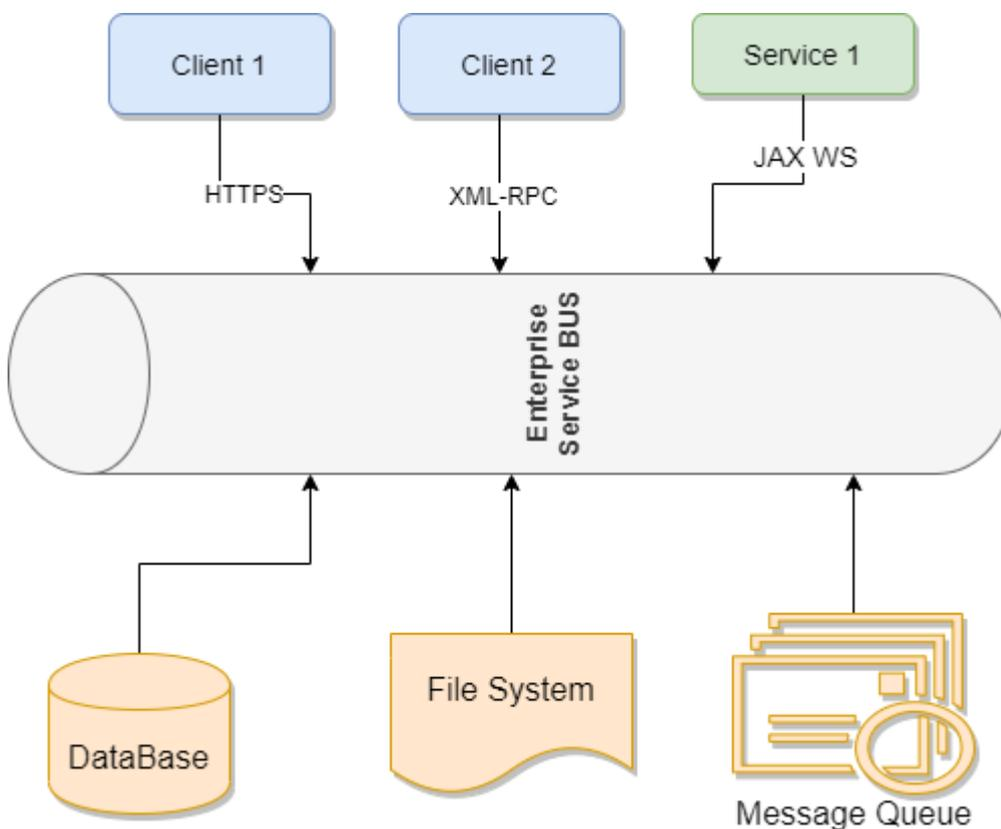
Service BUS: Service Oriented Architecture (SOA). It is based on loosely coupled components (services). Analogy of the BUS concept known in networks.
