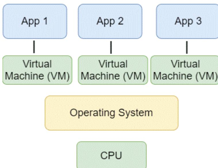
It has been widespread since the introduction of the Java VM (1997-). It defines a virtual processor and its associated so-called Byte Code, a set of instructions with its own machine code. It does not translate the source code directly to the CPU, but to the virtual machine's own byte code. Then VM converts the byte code to the machine code of the host system, when running. A virtual machine is usually a native application written in c/c++, which usually works on several platforms.
