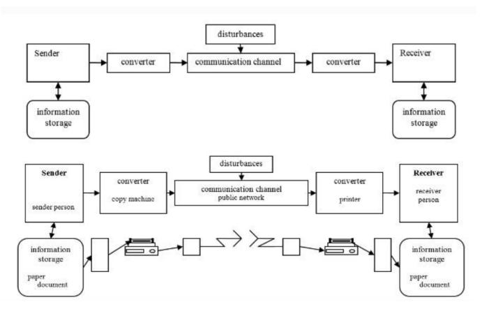
In the beginning the information is stored on a physical medium. The sender (person) converts it so therefore it can be transferred via the communication channel. This process is called encryption.
