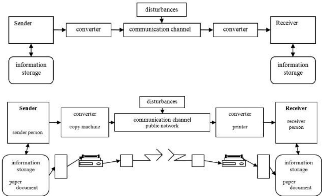
In the beginning the information is stored on a physical medium. The sender (person) converts it so therefore it can be transferred via the communication channel. This process is called encryption.
